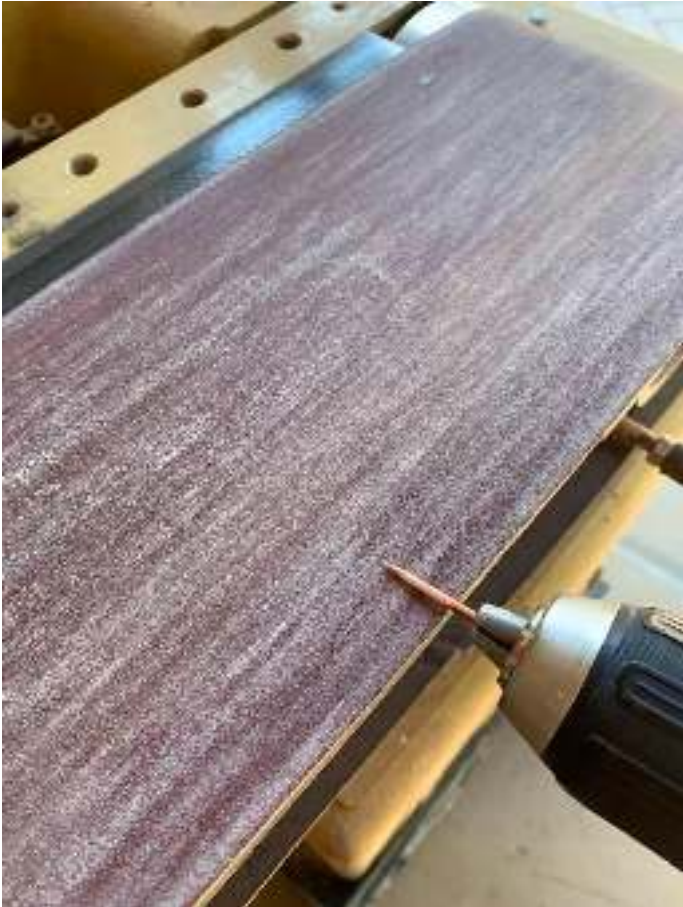
Shaping the toes out of 1/8" copper Wire
